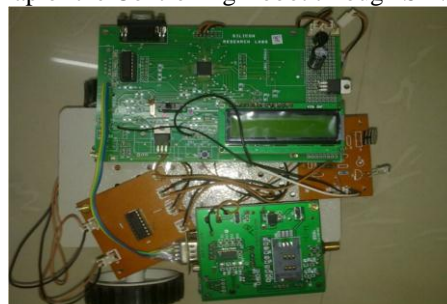
Figure 6. Controlling Robot through SMS with Acknowledging facility
