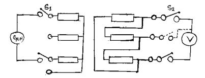
Figure 1: Single phase test, phase to phase Star - delta connected windings
