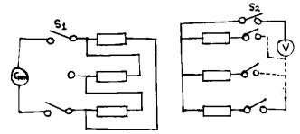
Figure 2: Single phase test, phase to phase Delta - star connected windings
