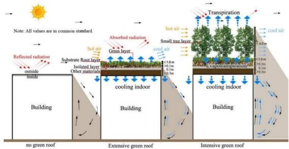
Figure 4.1a schematic structure of an extensive green roof and intensive green roof, and the cooling mechanism in the daytime.(Zhang, He, Zhu, & Dewancker, 2019)
