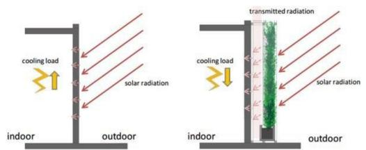
Figure 4.2. Difference between a conventional wall façade and a green façade. (Hadba, Silva, & Mendonca, 2017)
