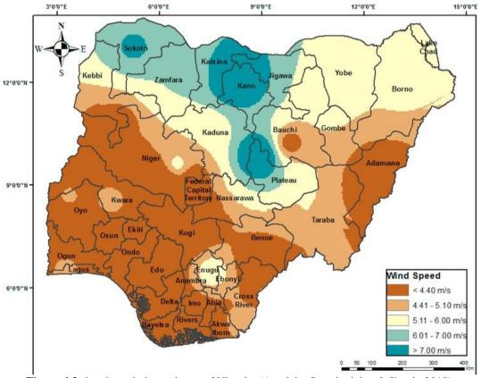
Figure 4.3 showing wind speed map of Nigeria. (Ayodele, Ogunjuyigbe, & Jimoh, 2018)
