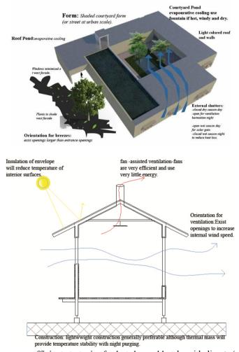
Figure 3.1.Showing energy efficient strategies for hot-dry and hot-humid climate 'rule of thumb 82-85' Adapted from (Heywood, 2013)
