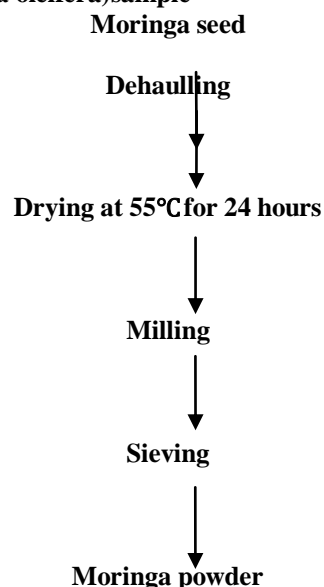
Fig 1: Flow diagram of moringa seed flour production
