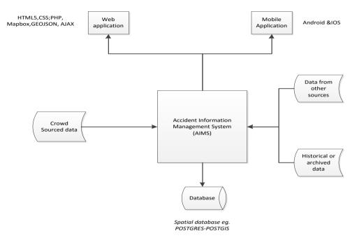
Figure 11: System Architecture
