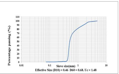
Figure 4.3: Particle Size Distribution of Imported Sand.
