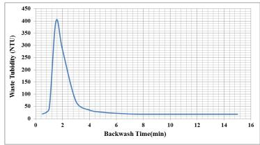
Figure 4.23: River CHANCHAGA Sand Bed Expansion at 26.5 %, Backwash Rate = 45.9 m/hr
