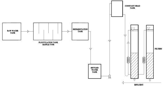
Figure 3.3: Schematic Diagram of Filtration Plant
