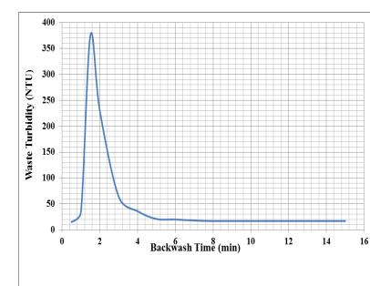
Figure 4.22: River Benue Sand Bed Expansion at 25.8 %, Backwash Rate = 45.9 m/hr
