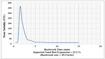
Figure 4.24: Imported Sand Bed Expansion at 22.2 %, Backwash Rate = 45.9 m/hr
