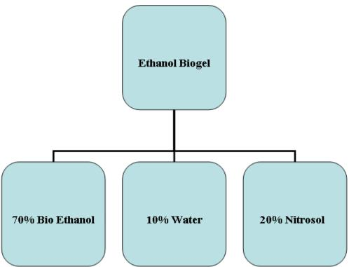
**Figure 2**: A flow diagram representing materials and formulation for production of ethanol biogel; an alternative source for cooking. Three ingredients as shown above were used for the production of the ethanol biogel. These are very much in abundance and thus describing the cheap production status and consistency of the product.
