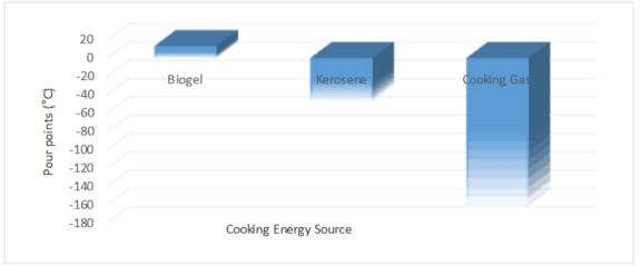
Figure 3b: Figure 2: Graphical representation of each cooking energy source pour point (°C)
