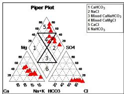
Fig.4.5. Piper Plot Showing Hydrochemical Facies
