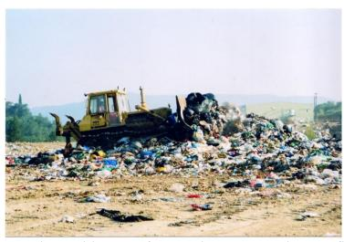
Fig 1: A bulldozer compacting municipal waste freshly delivered to the sanitary landfill site of Temploni on the island of Corfu. In the distance; the new Materials Recycling Facility (MRF) for processing commingled recyclables can also been seen (Author's photo)
