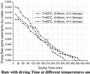
Fig. 6: Variation of Drying Rate with drying Time at different temperatures and velocity (1.5m/s) for slice thickness 6mm.
