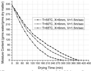
Fig. 2: Shows the effect of Temperature on the variation of the Moisture Content Vs Drying Time at 1.5 m/sec and slice thickness of 6 mm.
