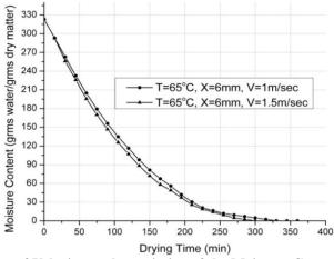
Fig. 3: Shows the effect of Velocity on the variation of the Moisture Content V/s Drying Time at Temperature 65°C for Slice thickness of 6 mm.
