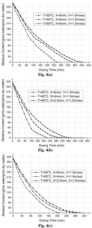
Fig. 4 (a, b and c) Shows the effect of Slice thickness (2.5mm, 4mm and 6mm) on the variation of Moisture Content V/s Drying time at different Temperatures 50°C, 60°C and 65°C for the Velocity 1.5 m/s.
