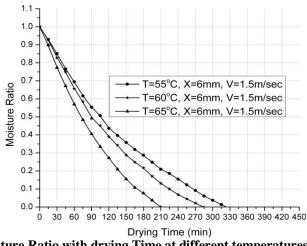
Fig. 5: Variation of Moisture Ratio with drying Time at different temperatures and velocity (1.5m/s) for slice thickness 6mm.
