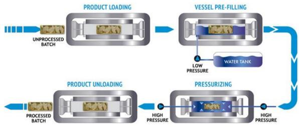
**Figure 1: Diagram of operation of HHP unit.** Source: <u>http://www.hiperbaric.com/en/hpp</u>
