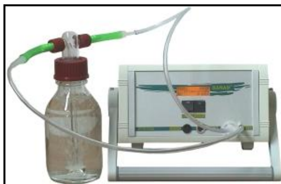
Figure2.Measurementconcentration of Radon 222 in the water by radon meter devicemodelRTM1688-2
