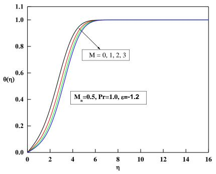
fig(6).Temperature profile  $\theta(\eta)$  versus  $\eta$  for different values of Melting parameter M.
