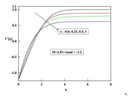
Fig(3).velocity profile f (  $\eta$  ) versus  $\eta$  for different values of magnetic parameter  $M_n$
