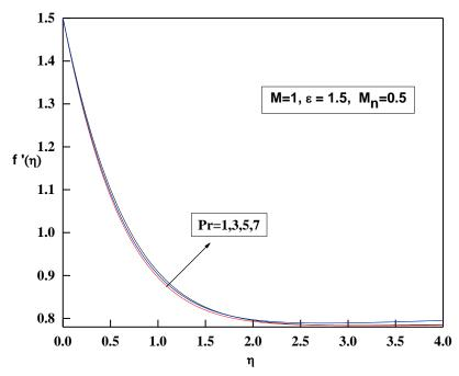
Fig(7). Velocity profiles f '( $\eta$ ) versus  $\eta$  for different values of Prandtl number Pr
