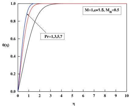
Fig(8). Temperature profiles  $\theta(\eta)$  versus  $\eta$  for different values of Prantdl number Pr.
