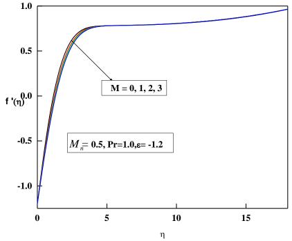
Fig(5). Velocity profiles f '( $\eta$ ) versus  $\,\eta$  for different values of Melting parameter M
