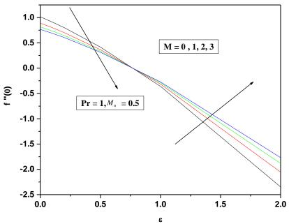
Fig(2) Variation of skin friction coefficient f  $^{\prime\prime}(0)$  with  $\epsilon$  for various values of M
