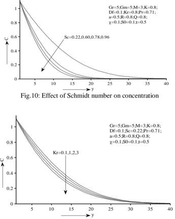
Fig.11: Effect of chemical reaction on concentration
