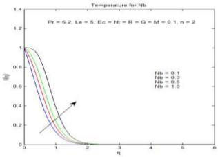
Figure 11 - Temperature profiles for Nb
