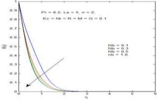
Figure 12 – Concentration profiles for Nb
