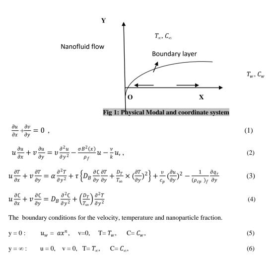
Here, u and v are the velocity components along the x and y axes, respectively.  $\alpha = k/(\rho c)_f$  is the thermal diffusivity,  $\sigma$  is electrical conductivity, v is the kinematic viscosity,  $\rho_f$  is the density
