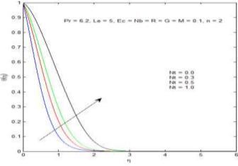
Figure 13 – Temperature profiles for Nt
