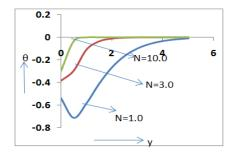
Fig6: Temperature profiles for different N when Gr=5.0,Pr=0.7,M=2.0,Gm=10.0,Sc=0.2,Sr=0.1, Du=0.45,S=1.0
