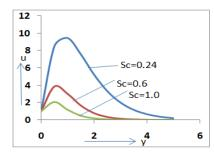
Fig5: Velocity profiles for different Sc when Gr=5.0, Pr=0.7,M=2.0,Gm=10.0,Sr=0.1 ,Du=0.2,S=1.0,N=1.0
