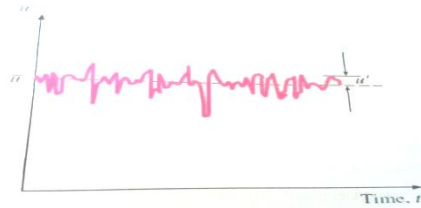
Figure 4: Fluctuations of the velocity component u with time at a specified location in turbulent flow.
