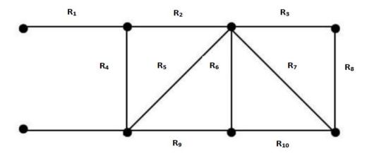
An undirected model representation of the circuit network with its edges is weight corresponding to the resistor value of each branch.
