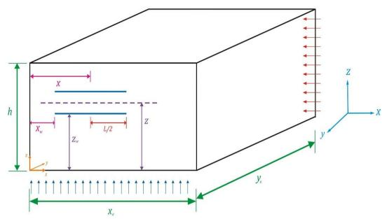
Figure 1: Horizontal well acting in an infinite reservoir
