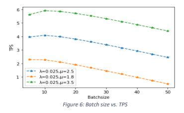
Figure 6 shows the graph of Batch size versus TPS. TPS indicates transactions per second i.e., throughput. It is observed that as batch size increases throughput decreases.
