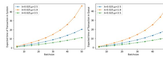
Figure 2: Batchsize vs. Expected transaction confirmation time
