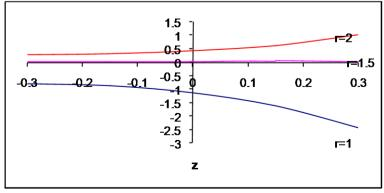
Figure 6: The radial stress function  $\sigma_{rr}/B$  in axial direction.
