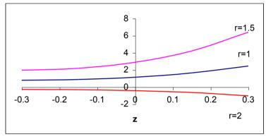
**Figure 8 :** The stress function  $\sigma_{\theta\theta}/B$  in axial direction.
