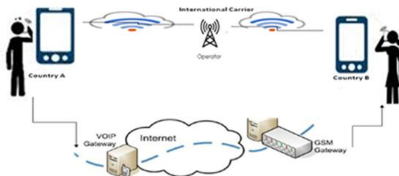
Fig 3. A unified Model of Bypass Structure
