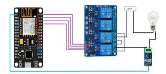
Connection established is Node MCU with Relay. The output signal of ACS712 sensor is connected with A0 pin of Node MCU. 2 channels of relay are connected in 3 way switching. This allow to control the load from any of two channels. With ACS712 connected, we can get to know if we are getting signal from channels or not.
