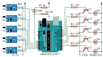
Figure no 7: Circuit diagramof the prototype
