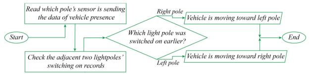
Figure no4: Direction of traffic determination
