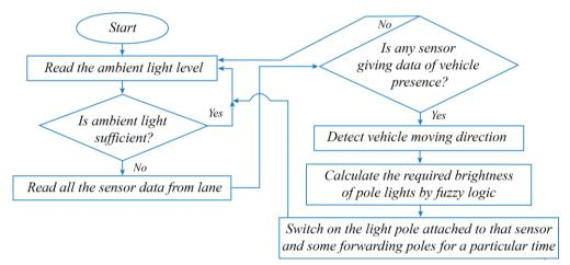
Figure no2: The algorithm of the intelligent streetlight system
