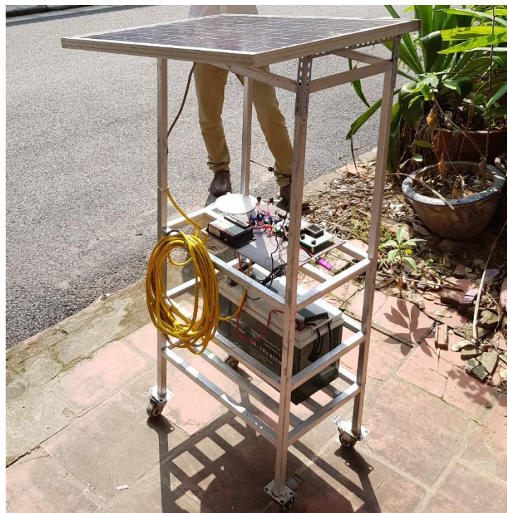
Figure5. Completed HPS model: solar panel, DC/DC solar charger, batteries and monitoring equipment
