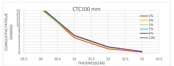
Fig. 3. Cumulative fatigue damage curve for Cement Treated Subbase (CTC) at different Subgrade strengths
