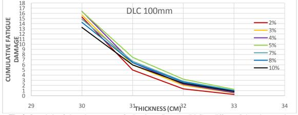
Fig. 2. Cumulative fatigue damage curve for Dry Lean Concrete (DLC) at different Subgrade strengths
