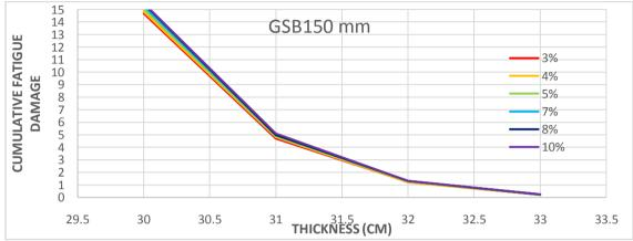
Fig. 1. Cumulative fatigue damage curve for Granular Subbase (GSB) at different Subgrade strengths
