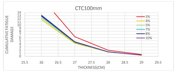
Fig.6. Cumulative fatigue damage curve for Cement Treated Subbase (CTC) at different Subgrade strengths
