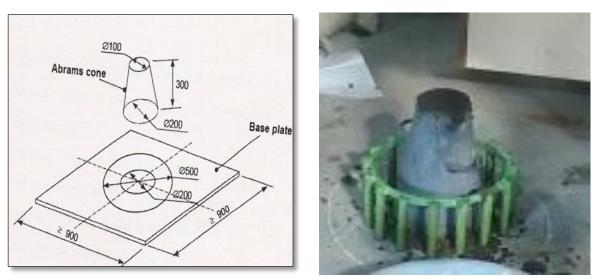
Fig 3.1 Slump Flow Test Apparatus
