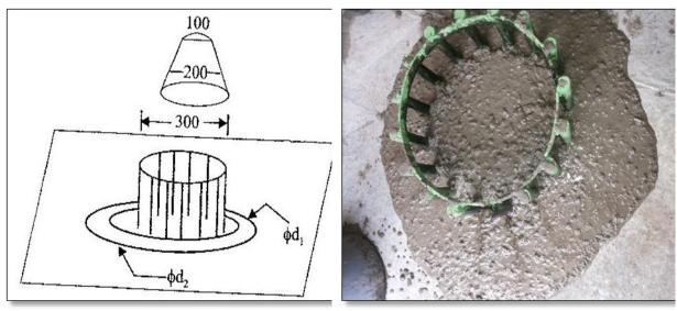
Fig 3.2 J-ring test apparatus
