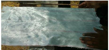
FIG.3.13 STRENGTHENED SLAB WITH GFRP
