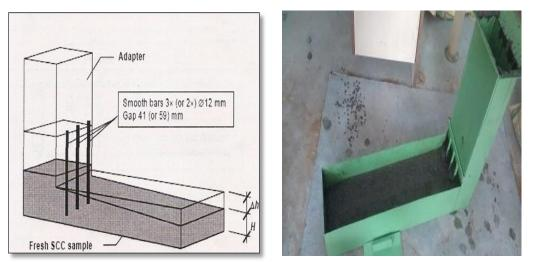
Fig 3.4 L Box Test Apparatus
