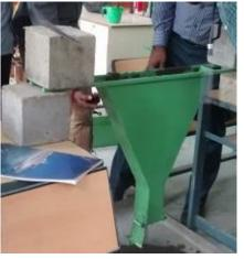
Fig 3.3 V-Funnel Test Apparatus
