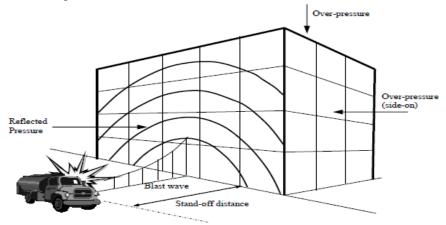
Fig.1 Blast Load effect on Building
