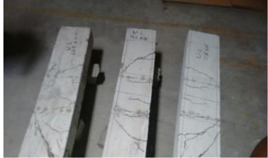
Fig 9 Crack pattern in beams
