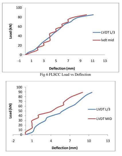
Fig 7 RC Load vs Deflection
