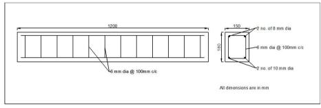
6.2a Reinforcement details as per IS13920
