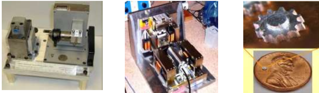
(a) Microturning machine (NWU). (b) Three-axis horizontal milling machine (UIUC). (c) Machined components
