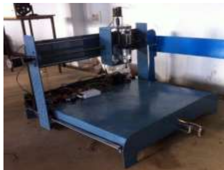
Fig.3: Fabricated Model of low cost CNC router [7]
