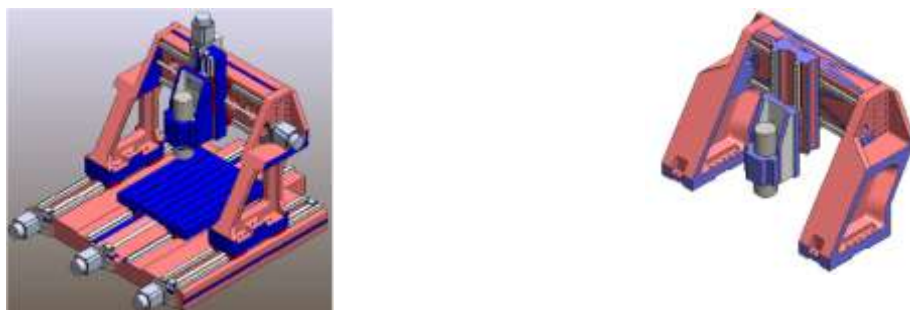
a) Preliminary Design of the gantry system b) Final Modified Gantry Structure Fig.10: Improvements in model of gantry [10]
