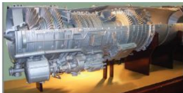
Fig: 5b Kaveri Engine Prototype with 2500 FDM parts
