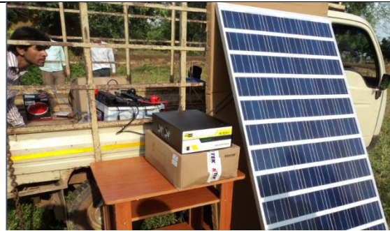
Fig 4: Parallel combination of animal power and solar power of 250W.
