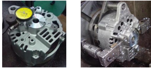
Fig 3.2 Bracket Machining and Parallelism Measurement
