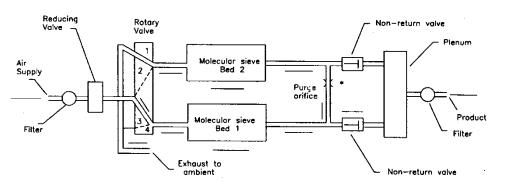
Fig.3 Typical two bed molecular sieve system
