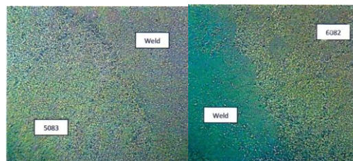
Figure 7 (a) Weld Interface between Weld zone and Base metal AA 5083 (b) Weld Interface between Welds Zone and Base Metal AA 6082
