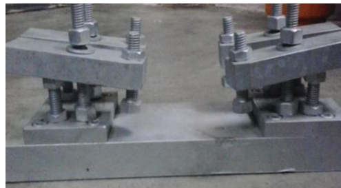
Figure 3 Friction Stir Welding Fixture
