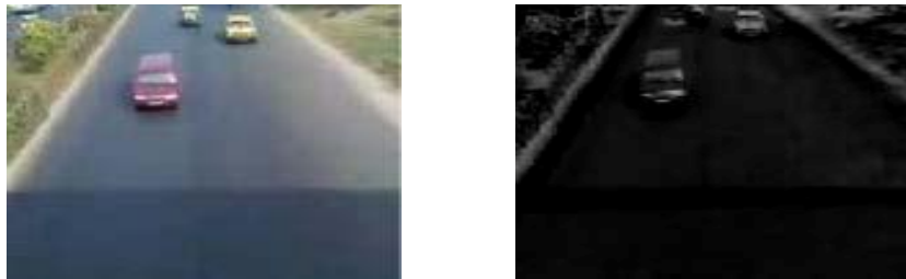
Fig.1.a Color image from real time video, 1.b after background Subtraction
