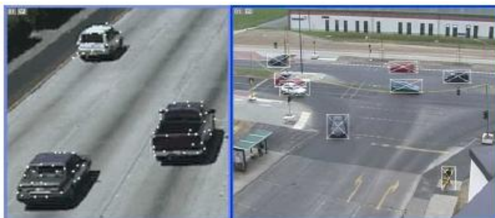
Fig 5. Left: An enlarged picture showing detected corners of vehicles marked by white dots. Right: Bounding boxes of moving vehicles and their centers marked by white crosses.
