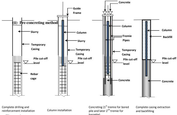
**Figure 4:** General construction sequence of pre-concreting installation method In this method, column is installed immediately after completion of drilling and reinforcement lowering prior to concreting process. In some projects column is attached to the last section of reinforcement and installed.
