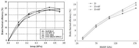
Figure-3 Variation of BTE with BMEP with respect to engine load at 2200 rpm
