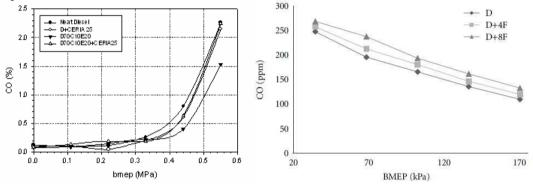
Figure-4 Variation of CO with BMEP with respect to engine load at 2200 rpm The CO emission is marginal up to the BMEP of 0.44 MPa and then increases rapidly with higher load. The
