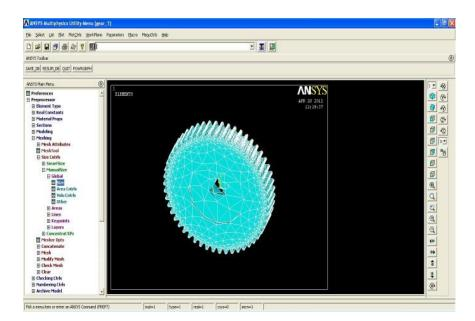
Figure No. 1 Meshing of Gear
