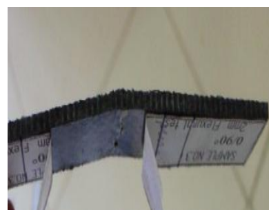
Fig.9 Fractured Flexural Specimen
