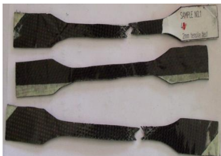
Fig.8 Fractured Tensile Specimens
