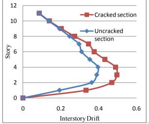
Fig.16 Interstory Drift for uncracked and cracked section for Push-Y b) For uncracked section with different position shear wall in y-direction For Push-X Direction
