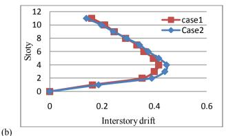
Fig.22 Interstory Drift for Cracked section with different Position of shear wall in x-direction for Push-X (a) Push-Y (b)
