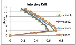
Fig.17 Interstory Drift for uncracked section with different position of shear wall in y-direction for Push-X
