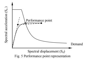
Check performance level of the structure and plastic hinge formation at performance point. A performance check verifies that structural and non-structural components are not damaged beyond the acceptable limits of the performance objective for the force and displacement implied by the displacement demand.
