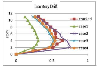
Fig.19 Interstory Drift for Cracked section with different Position of shear wall in y-direction for Push-X **For Push-Y Direction**
