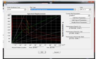
Fig.14 Capacity Spectrum Curve
