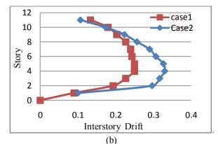
Fig.21Interstory Drift for Uncracked section with different Position of shear wall in x-direction for Push-X (a) Push-Y (b)
