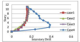
Fig.18Interstory Drift for uncracked section with different position of shear wall in y-direction for Push-Y
