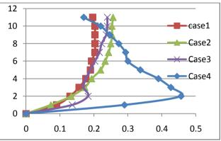
Fig.20 Interstory Drift for Cracked section with different Position of shear wall in y-direction for Push-Y
