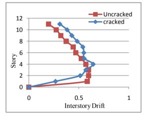
Fig.15Interstory Drift for uncracked and cracked section for Push-X
