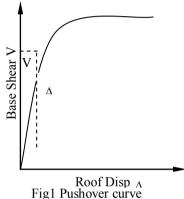
In order to use the Capacity Spectrum Method, it is necessary to convert the capacity curve obtained from pushover analysis in terms of base shear, V and roof displacement  $_{\Delta}$ , to the capacity spectrum (Fig.2). Capacity spectrum is the representation of the capacity curve in ADRS (Acceleration Deformation Response Spectrum) format. This transformation can be done by using Equation 1 and Equation 2.
