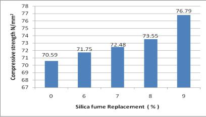
Fig. 2. Variation of Compressive Strength with Silica fume percentage
