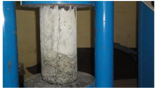
Fig .1 Compressive strength of cylinder load set up
