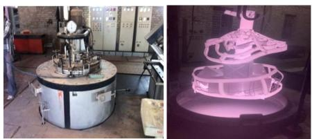
Figure 1. Electric Furnace Figure 2. Hot Cubes Being Taken Out Of Furnace
