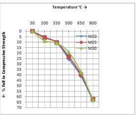
Figure 5: % Fall in compressive strength after 1 hour Figure 6: % Fall in compressive strength after 2 hours
