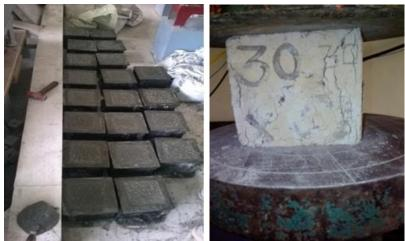
Figure 3: Casting of Cubes
