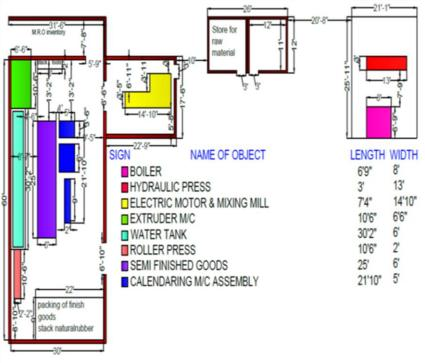
Fig 6 Existing Plant Layout of C.R.P at G.I.D.C
