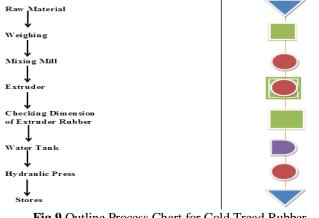
Fig 9 Outline Process Chart for Cold Tread Rubber
