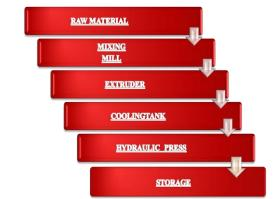
Fig 5 Manufacturing Sequence for Cold or Pre-cured Tread Rubber
