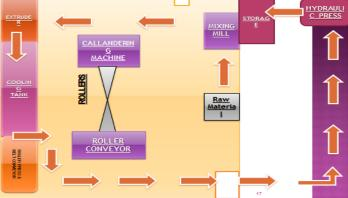
Fig 4.Material Flow of Cold or Pre-cured Tread Process
