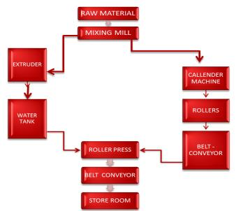
Fig 3 Manufacturing Sequence for Hot or Conventional Tread Rubber
