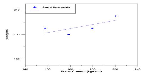
Figure 01: Relationship between Slump of control mix and water content
