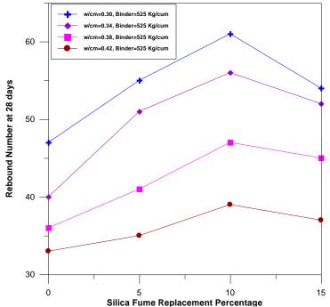
Fig 01: The relationship between rebound number and silica fume replacement percentages
