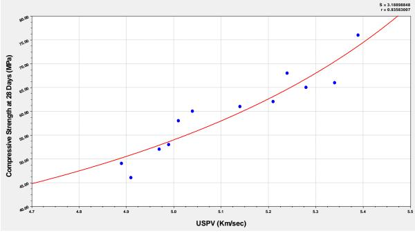
Fig 06: The relationship between compressive strength and uspv for silica fume mixes:
