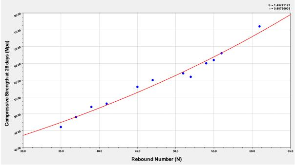
Fig 03: The Relationship between rebound number and compressive strength for silica fume mixes.
