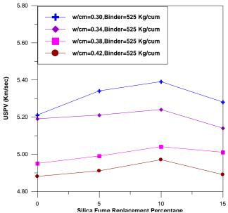
Fig 04: The relationship between uspv and silica fume replacement percentage
