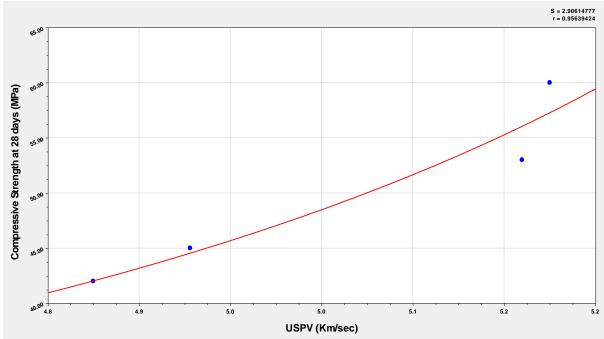
Fig 05: The relationship between compressive strength and uspv for control mixes.
