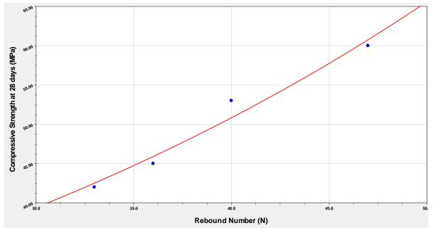
Fig 02: The Relationship between rebound number and compressive strength for control mixes.
