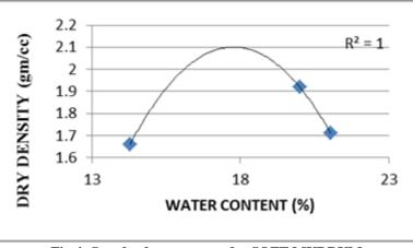
Fig.4: Standard proctor test for SOFT MURRUM
