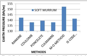
Fig.12: Earth pressure of soft murrum for different Method
