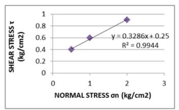
Fig.9: Direct shear test for BLACK COTTON SOIL
