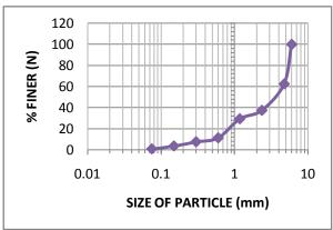
Fig.3: Gradation curve for BLACK COTTON SOIL
