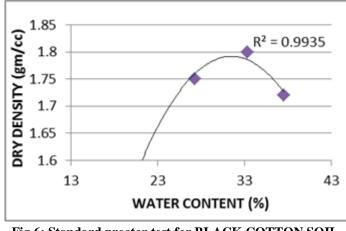
Fig.6: Standard proctor test for BLACK COTTON SOIL
