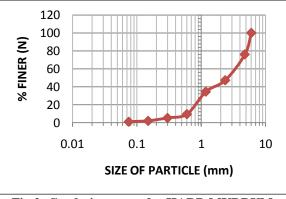
Fig.2: Gradation curve for HARD MURRUM
