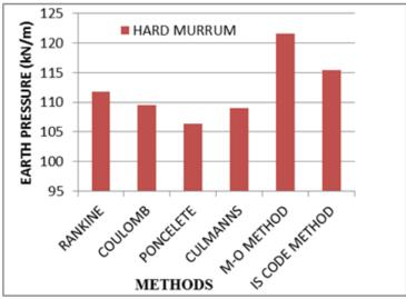
Fig.13: Earth pressure of hard murrum for different Method
