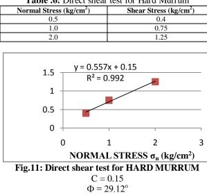
Table .6: Direct shear test for Hard Murrum
