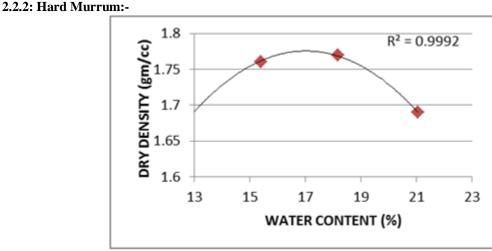
Fig.5: Standard proctor test for HARD MURRUM
