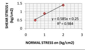
Fig.8: Direct shear test for HARD MURRUM
