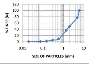
Fig.1: Gradation curve for SOFT MURRUM
