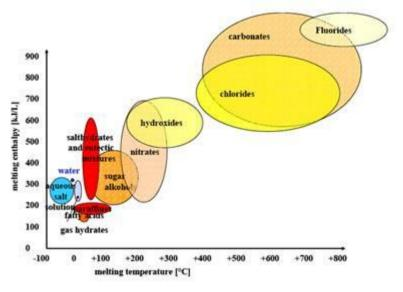
**Fig. 2.3:** Melting enthalpy of various phase change material groups in relation to their melting temperature [5]
