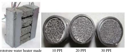
Schematic of prototype water heater made10 PPI20 PPIof open cell aluminum and heateropencell aluminum of 10, 20 and 30 PPI
