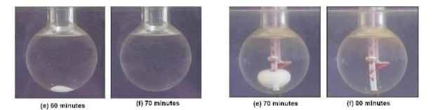
For the unconstrained melting, the solid PCM sinks to the bottom of the sphere. This is due to heavier density of the solid PCM than the liquid PCM. Under the same experimental condition, unconstrained melting seems to occur at a faster rate than the constrained melting. This is due to larger rate of heat transfer by conduction from the solid PCM to the spherical glass capsule [21].
