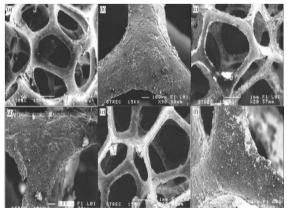
SEM micrographs showing structures of pure AC3A and composite foams containing 1% and 5% SiC particles: (a), (b) PureAC3A; (c), (d) AC3A+1%SiC; (e), (f) AC3A+5%SiC
