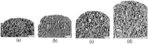
Product of foam with different fraction of SiCp (12µm) a) %5, b) %10, c) %15, d) %20
