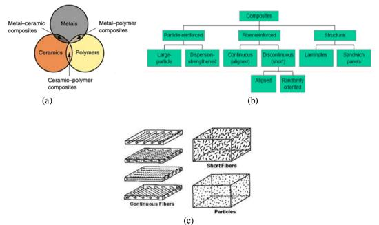
Figure (3.1): a- Classification of composites by matrix type, b- Classification of composites by filler type and c-examples of composite reinforcements.
