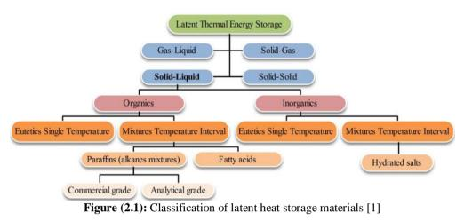
The storage capacity of the phase change materials is equal to the phase change enthalpy at the phase change temperature + sensible heat stored over the whole temperature range of the storage (Fig. 2.2). The PCM continues to absorb heat without a significant rise in temperature until all the material is transformed to the liquid phase. When the ambient temperature around a liquid material falls, the PCM solidifies, releasing its stored latent heat [2].
