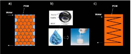
a. Macro-encapsulation, b. Micro-encapsulation ,PCM slurries, c. PCM in tank, immersed heat exchanger Fig. 2.4: Integration of phase change materials into (TES), [9]
