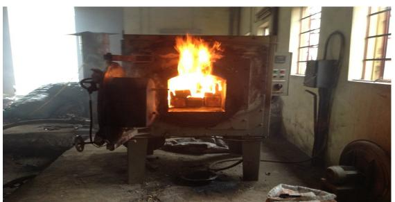
Fig. 3: Burning specimen inside furnace after expiration of 1-hour fire exposure
