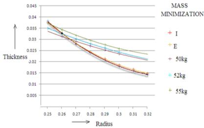
Fig.1.Graphical Representation of Mass Minimization of Solid Disk Flywheel
