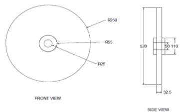
Fig.2.Optimal Solid Flywheel
